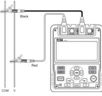
Figure 4. Voltage Measurement
