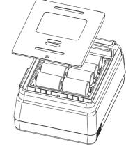
Figure 8. Battery Replacement
