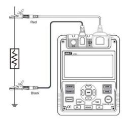
Figure 5. Insulation Resistance Measurement
