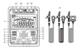
9 10 11 Figure 1. The Meter Front Structure
