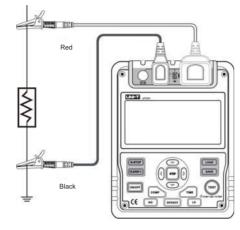
Figure 6. Low Resistance Measurement
