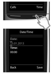
Press the key Time below the display screen to open the input field.
